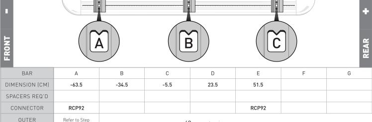
OUTER Refer to Step 11-12 in the UNDERBAR Pioneer Series 6 COVER Instructions to trim (mm/in) B and C CENTRE Refer to Step 11-12 in the UNDERBAR Pioneer Series COVER 6 Instructions to (mm/in) trim A
